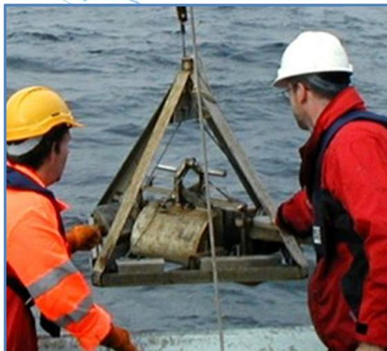
A further extended bucket lip reduces sediment washout during retrieval. The unit can be supplied with a stand allowing for easy sample access and handling. A further modification that was made provided an efficient closure system to allow arming by a single person. This modified Day grab has become the standard operating tool for the North Sea.
